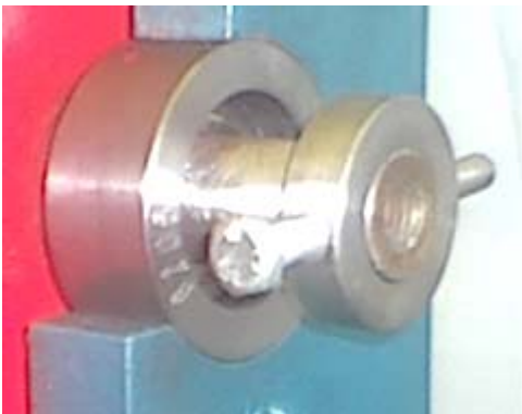
Figure 2 - Spin drive coupling cylinder side
