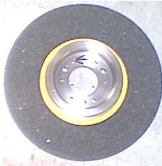
Figure 52 – Mark one of the balancing holes
