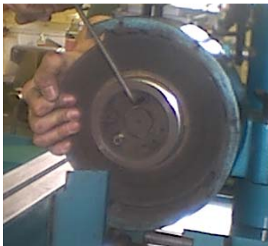
Figure 51 – Removing the wheel securing flange
